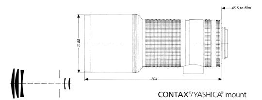
The 300 mm Tele-Tessar® T\* f/4 lens offers a long focal length, remarkably high speed, compact design and easy operation at one and the same time. It is a telephoto design where the distance between the front lens vertex and the rear focus is only about 80% of the focal length. It offers virtually perfect monochromatic correction and excellent image quality even at full aperture - a decisive improvement over earlier telephoto designs.
